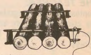
A RAFT CAN BE EASILY BE MADE BY LASHING LOGS TOGETHER.
